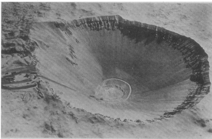
Fig. 1. Sedan Crater, Yucca Flat, Nevada Test Site, Nye County, Nevada (view is to the north-northeast). Crater diameter is 370 m, depth 98 m, and volume 5.0 \times 10^6 \text{ m}^3 . Crater formed in 1962 by a 100 \pm 15 kiloton nuclear device detonated at a depth of 190 m in valley fill. Water table is about 580 m below land surface. Vehicles, left side of photo, provide scale. [Photo from W. D. Richards (11)]
