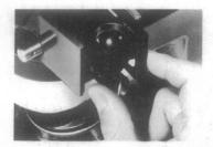
Matched and precisely aligned barrier, exciter and dichroic filter combinations in interchangeable Fluor Clusters make AO fluorescence more convenient and faster. All AO FLUORESTAR® One-Ten and One-Twenty microscopes have this advanced filter system. A flip of a lever positions the desired filter combination. The same lever switches the microscope to transmitted brightfield.
