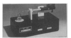
tain" and "to deliver" models are monitored easily. The large evaporative error inherent in gravimetric methods is eliminated, especially in small volumes. The VC-100 includes a digital microburet and a combination mixing-delivery system. Required reagents and disposables are also available. Streck Laboratories. Circle 816.
