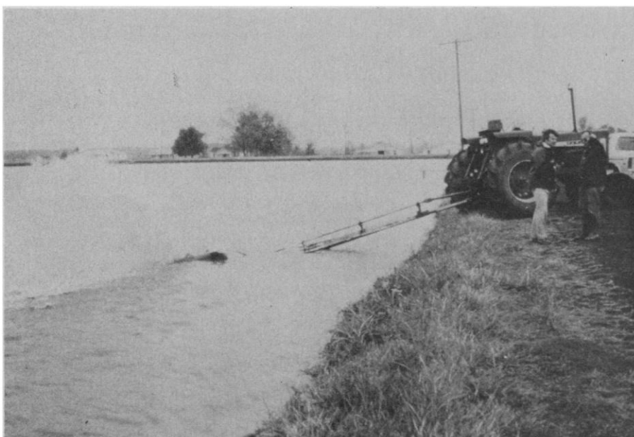
Fig. 2. Emergency aeration by tractor-mounted paddlewheel of an oxygen-depleted catfish culture pond. The fish swim to the oxygenated water near the aerator and remain until the pond recovers.
