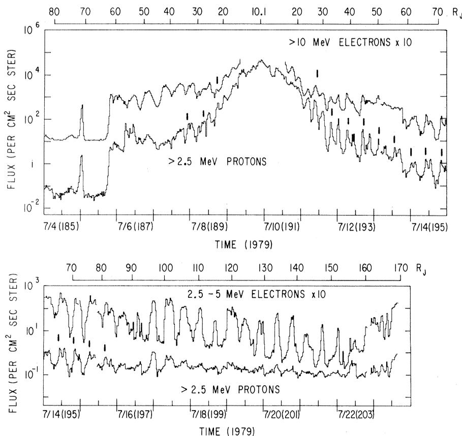
Fig. 1. Electron and proton fluxes (32-minute averages) observed during the Voyager 2 encounter. Electron fluxes are 1/10 of the left scale. Proton flux maxima corresponding to magnetic equatorial crossings in the active hemisphere have been identified with tick marks.
