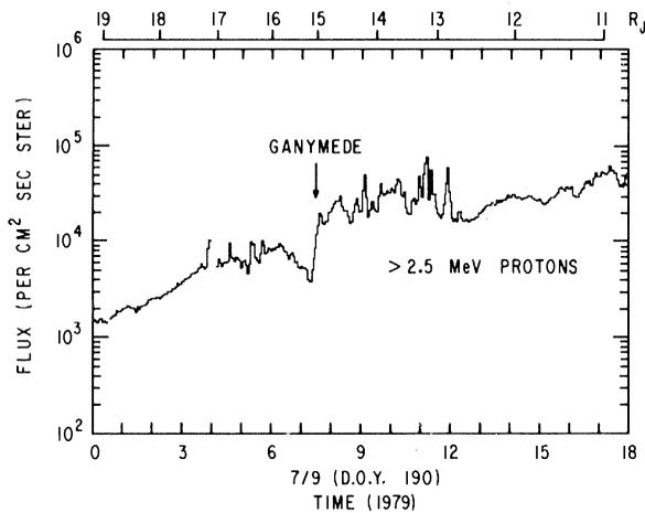
Fig. 2. Approximate intensity of protons with energies above 2.5 MeV (3.2-minute averages) observed during the inbound pass between 19 and 11  $R_J$ . Note the large intensity fluctuations at  $15 \pm 2 R_J$ , which fall within  $\pm 4$  hours of the closest approach to Ganymede.
