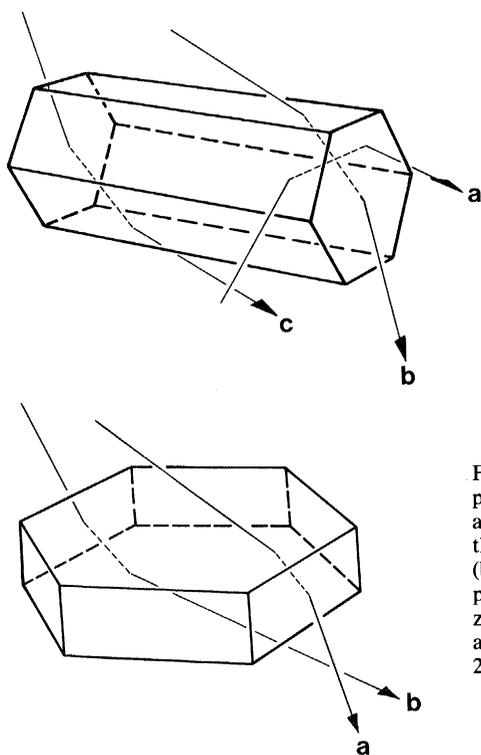
Fig. 1 (top left). Light rays passing through a pencil ice crystal. Ray a results in the  $22^\circ$  halo and its associated arcs; rays b and c result in the  $46^\circ$  halo and its associated arcs. Fig. 2 (bottom left). Light rays passing through a plate crystal. Ray a results in the circumzenithal arc; ray b, the circumhorizontal arc. Fig. 3 (top right). Simulation of the  $22^\circ$  and  $46^\circ$  halos.
