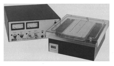
That's how easy it is with LKB's Multiphor® unit. And duration of the runs is also short: the precisely engineered all-glass cooling stage means that you can apply higher power for faster runs higher field strengths for sharper resolution. With the Multiphor unit and LKB's power supply you can do up to 48 samples in less than two hours!
