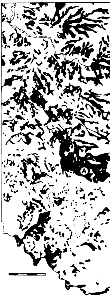
Fig. 2. Diagram of a portion of an aerial photograph taken 3 days after the earthquakes occurred showing the patchiness of landslides within the highly damaged central area. Black areas are landslides, dashed lines represent clouds on the photograph, and A is an approximately 100-ha denuded area. The irregular lower edge is the Pacific coastline. The top is north, and the scale bar represents 1 km.
