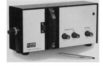
Sensitivity is increased up to 200x for proteins when you monitor at 206 nm with LKB's new Uvicord® S UV-monitor. This unique instrument will detect non-aromatic peptides, polysaccharides, nucleotides, lipids and steroids as well as proteins. And, naturally, you can also monitor at 254 or 280 nm.
