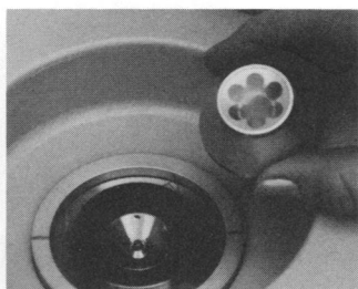
The stator pad has vertical jets to levitate the rotor. Driving jets take the rotor to full speed in 30 seconds.
