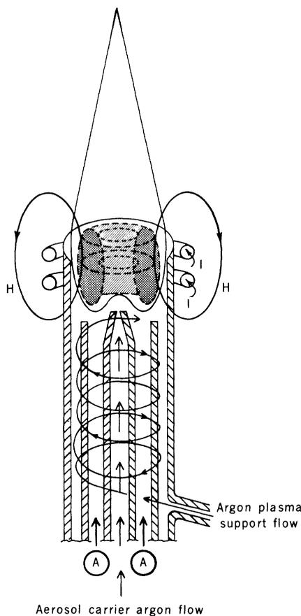
Fig. 2. Typical inductively coupled plasma configuration (11).
