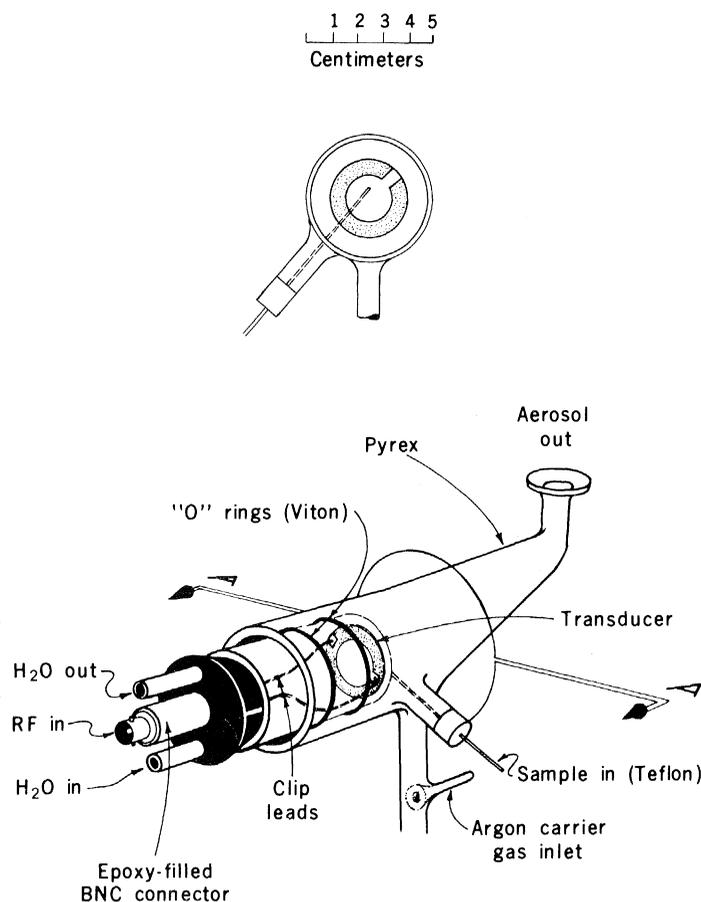
Fig. 4 (right). Ultrasonic nebulization facility (16).
