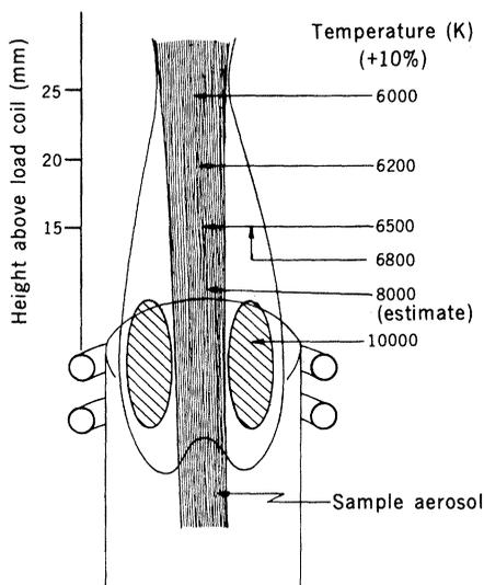
Fig. 5 (left). Schematic diagram of sample flow through the plasma and the temperatures experienced (11).
