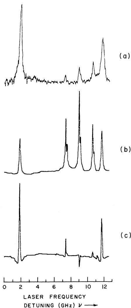
Fig. 7. Fine structure of the hydrogen  $H_{\alpha}$  line obtained by (a) saturated absorption with a pulsed dye laser, (b) saturated absorption with a continuous-wave dye laser, and (c) polarization spectroscopy with a continuous-wave dye laser. [Courtesy of J. E. M. Goldsmith, E. W. Weber, and T. W. Hänsch]
