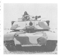
The chief new feature of the XM-1 is its method of protection, a material of classified composition known as Chobham armor after the location of the British research unit where it was invented (*Science*, 14 July 1978). The 105-mm cannon and the smoke grenades are also of British design.
