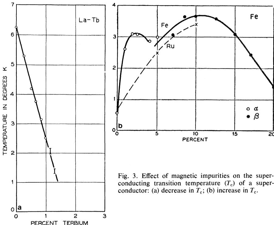
Fig. 3. Effect of magnetic impurities on the superconducting transition temperature ( $T_c$ ) of a superconductor: (a) decrease in  $T_c$ ; (b) increase in  $T_c$ .
