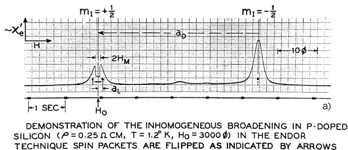
Fig. 11. (a) Hole-digging and ENDOR spectrum. While saturating a specific frequency (a) a radio-frequency signal of variable frequency is applied (b). Note the slow refilling of the hole (exponential recoveries) in (b): the sweep time is several minutes. This is the  $^{29}\text{Si}$  spin-lattice relaxation, enhanced by the radio frequency applied.
