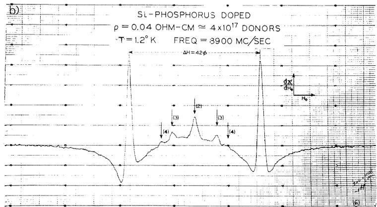
Fig. 10. (a) Hyperfine structures of donor electron paramagnetic resonance at increasing donor ( $P$ ) concentrations through the Mott-Anderson metal-insulator transition. (b) Example of well-developed cluster lines.
