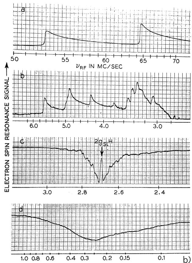
DOUBLE RESONANCE SPECTRUM IN P-DOPED SI.  $\approx 2 \times 10^{16} \text{ P/CM}^3$ ,  $T = 1.3 \text{ K}$ ,  $\nu_e \approx 9000 \text{ MC/SEC}$
