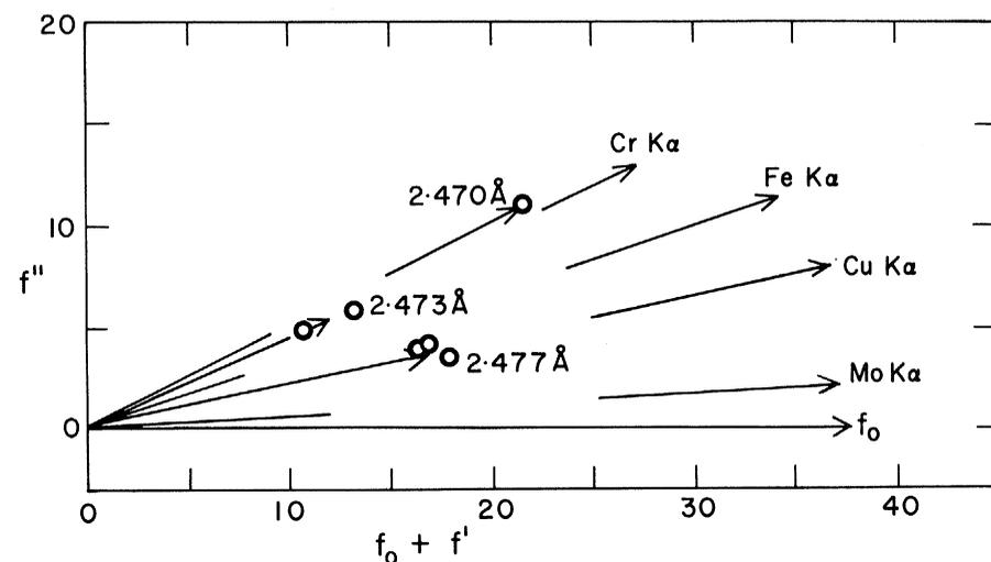
Fig. 2. Atomic scattering vectors for cesium for  $(\sin\theta)/\lambda = 0.3 \text{ \AA}^{-1}$ , where  $f_0 = 38$ . The length of each vector represents the amplitude of the wave scattered by the atom, and the angle from the horizontal represents the phase shift relative to scattering by a free electron. The circles represent our experimental points. The other vectors are calculated (8) for some wavelengths available from conventional x-ray tubes.
