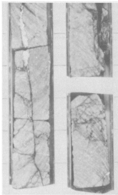
Fig. 1. Core (8 centimeters in diameter) of fractured crustal rock recovered from 110-million-year-old ocean crust. Filling of natural cracks by carbonates (white) and smectite clays (gray) occurred in the presence of flowing seawater. [Source: Douglas Johnson, University of Texas at Dallas]
