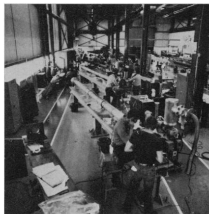
Fig. 2. View of the production line at the Fermi National Accelerator Laboratory for producing long superconducting dipole magnets for the energy doubler/saver project.
