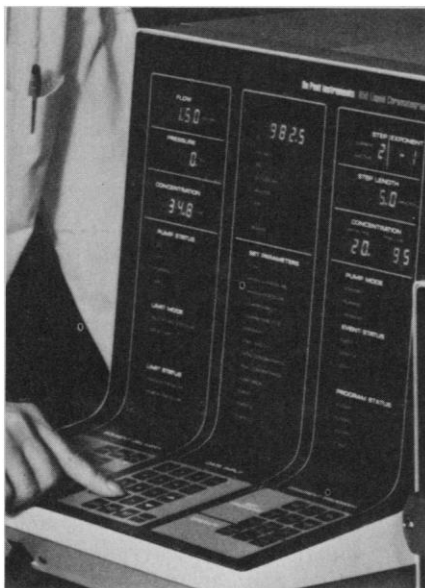
Fig. 1. The DuPont model 850 HPLC features heat-sensitive switches and a flush control panel.
