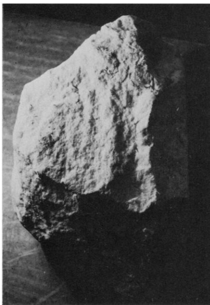
Fig. 3. Sample EM 6958. A strong lineation by fold axes that run from top to bottom and parallel to the direction of lettering on the face is seen on the back. The stone is 22 cm wide.
