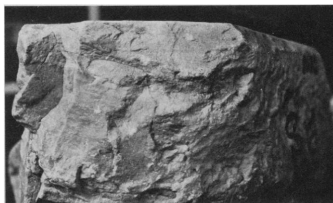
Fig. 1. Sample EM 8682, oriented with the top to the viewer. The stone is 18 cm thick. Color variation in bluish grays makes up the planes of layering, dipping to the right for EM 8682 (shown) and to the left for EM 8680 (not shown).
