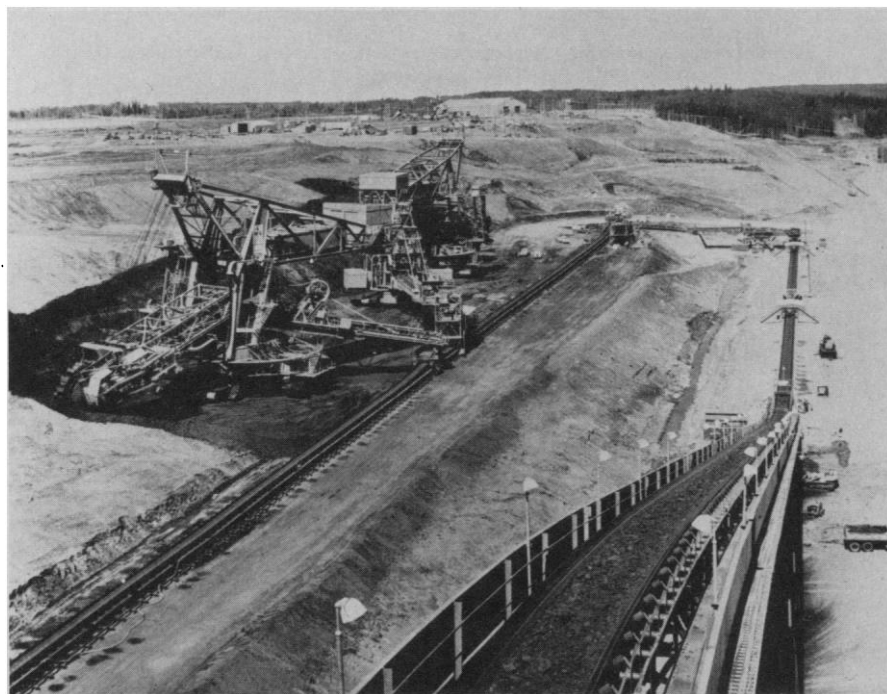
Fig. 2. These two bucket wheel excavators at GCOS load 108,000 tons of tar sands onto the conveyor belt each day. Note the size of the bulldozer and trucks in the lower right foreground. [Source: Sun Company Inc.]
