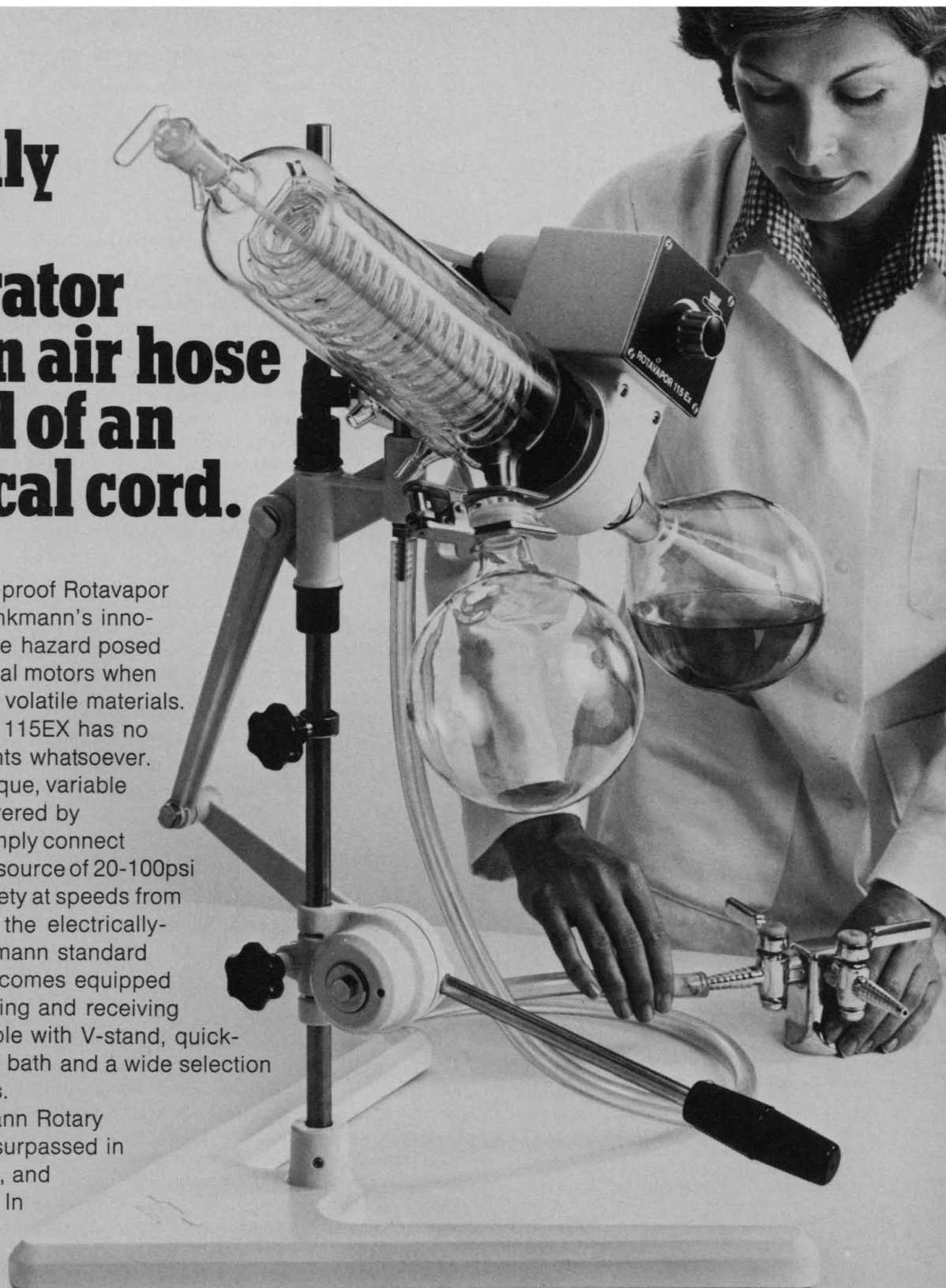
ROTAVAPOR R-175EX For 20-liter volumes. Explosion-proof motor.
