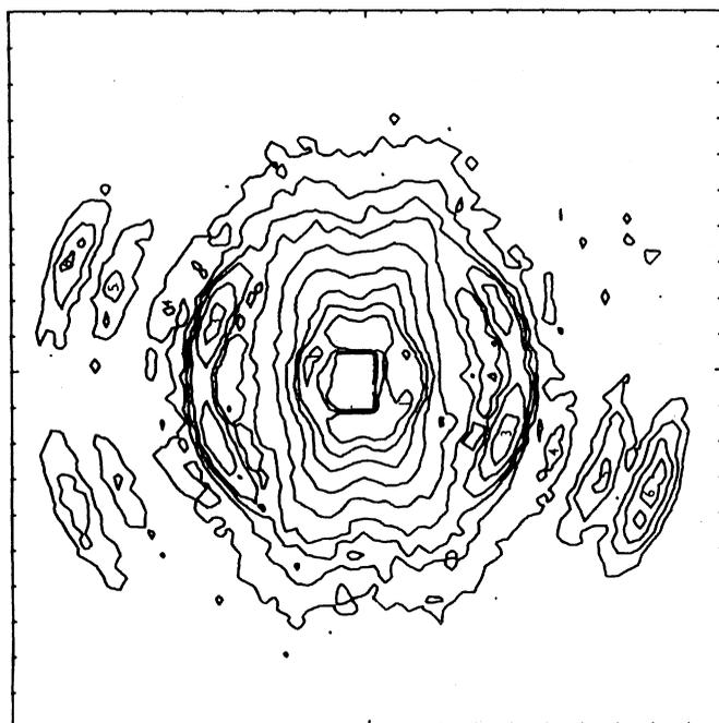
Fig. 3. Low-angle neutron diffraction pattern from a dissected sheet of annulus fibrosus immersed in a  $\text{D}_2\text{O}$  solution of 0.15M NaCl. The specimen-detector distance was 2.82 m and the wavelength of incident neutrons 11.1 Å.
