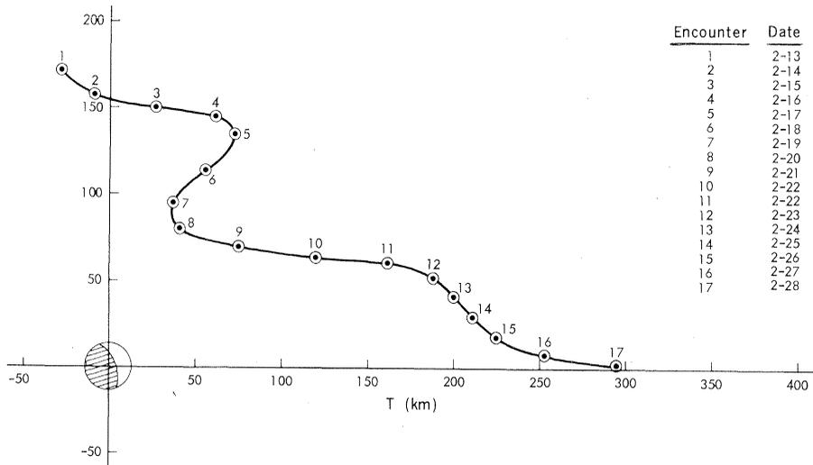
Fig. 3. The distance of VO-1 to Phobos is shown for each flyby (one flyby per ~23 hours). The view is as would be seen as VO-1 approached Phobos with the  $T$  axis parallel to the martian equatorial plane. A closest flyby distance of 88 km was achieved on 20 February 1977. All flybys were within 300 km during this 2-week encounter period.
