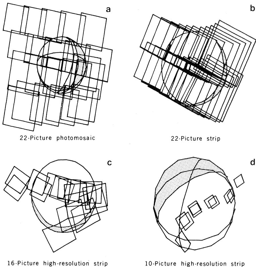
Fig. 4. Four basic television picture sequences were used to image Phobos near encounter: (a) and (b) were taken at range greater than 400 km to completely cover Phobos; (c) and (d) were taken to obtain higher resolution at the expense of coverage.
