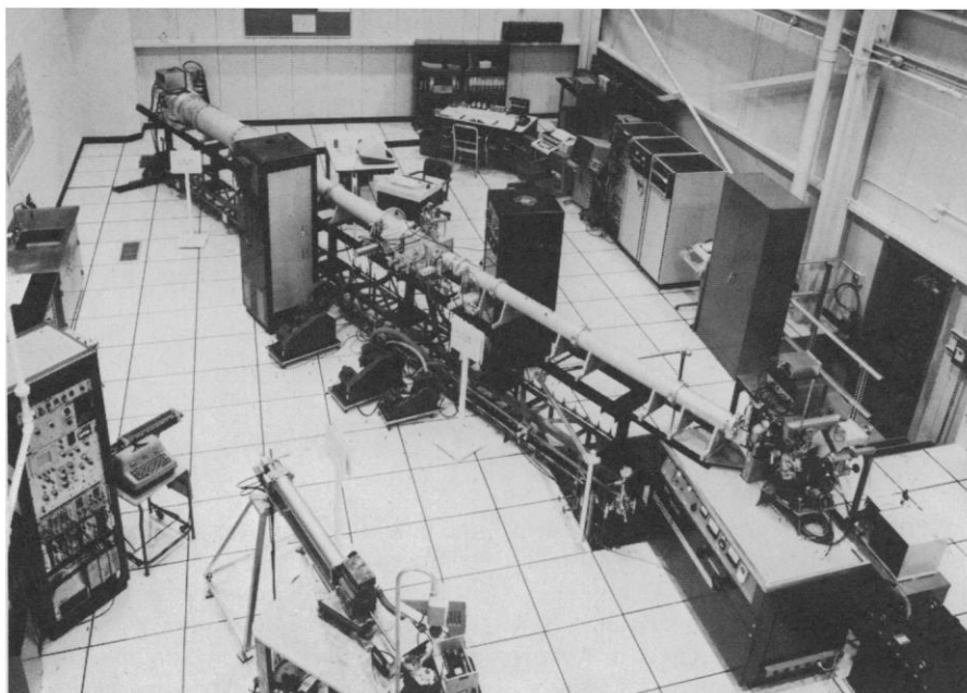
Fig. 2. Small-angle x-ray scattering facility at the Oak Ridge National Laboratory. A rotating anode x-ray source is at the right end of a 10-meter long evacuated tube. The length of the tube depends on the requirement that angles less than 0.1^\circ be resolvable by the detector, whose spatial resolution is better than but still limited by the spacing between the wires in the anode and cathode arrays. Specimens are mounted in the box near the center of the tube. The position-sensitive detector is at the far left end of the tube. In the right rear corner are the minicomputer and other electronics devices for controlling and monitoring operation of the experiment. [Source: R. W. Hendricks, Oak Ridge National Laboratory]
