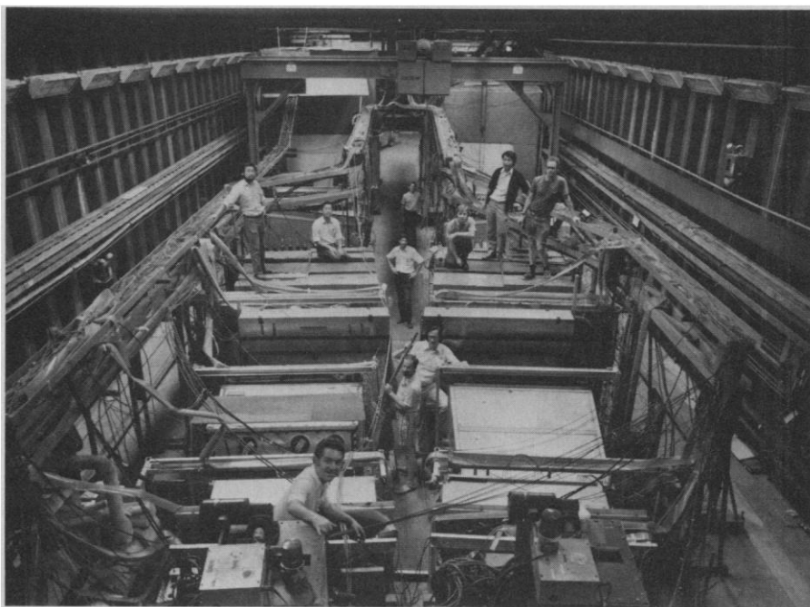
Fig. 1. Detector used by Lederman's group at Fermilab to record pairs of muons. Collisions between 400-GeV protons and a copper-platinum target takes place out of sight in the foreground. Shown are symmetric arrays of magnets, charged particle detectors, and steel absorbing blocks to select out the highly penetrating muons. [Source: Fermi National Accelerator Laboratory]
