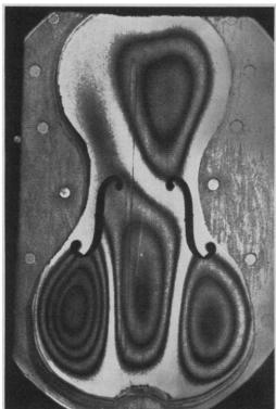
These are hologram reconstructions, photographs made with a camera receiving images originally recorded as time-average interference holograms. The dark fringes connect all points of common amplitude on the inside of the vibrating top of an experimental viola. It's part of an effort to improve the loudness, dynamic range, and playing ease of the viola.
