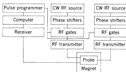
Fig. 1. Block diagram of an NMR spectrometer.
