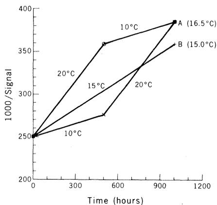
Fig. 2. A hypothetical example illustrating a difference in accumulated fade due to a fluctuating (A) and a uniform (B) average temperature exposure of  $15^\circ\text{C}$ . The anticipated TL signals were calculated on the basis of previously determined fade rates for the temperatures indicated. The calculated average temperatures (based on the final TL signal) are given in parentheses.
