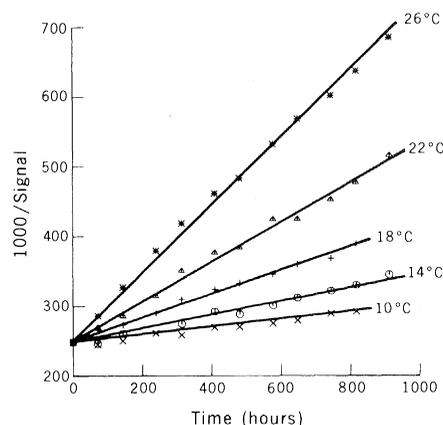
Fig. 1. Isothermal fade response observed for  $\text{CaSO}_4:\text{Mn}$  tags at the five temperatures indicated. Data points are the mean TL signal for one tag and have a 3 percent standard error at the 95 percent confidence level. Lines were fitted to the data by a combined computer analysis that specified both a hyperbolic fade response and a fixed relationship between fade rate and temperature.
