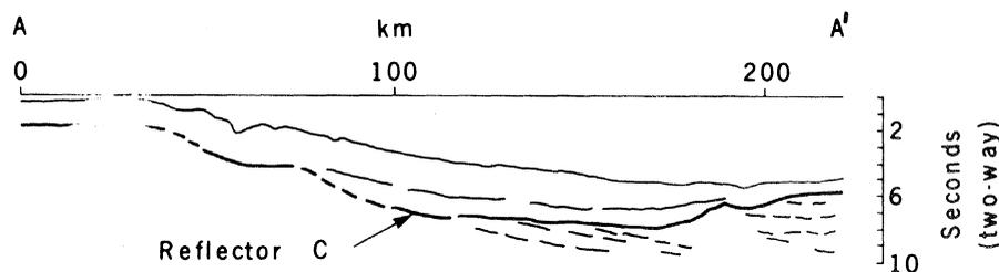
Fig. 5. Line drawing of a multichannel reflection seismic profile extending from the southern Grand Banks to the J-anomaly ridge (see location in Fig. 1).
