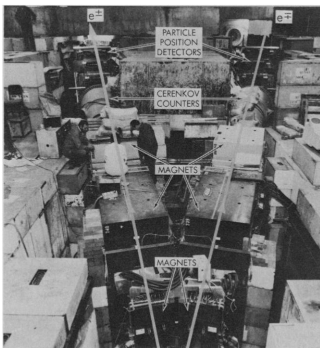
Fig. 8 (left). Overall view of the detector. Fig. 9 (right). End view of one arm, showing part of the Čerenkov counter C_e and the chambers A, B, C, with part of the 8000 amplifiers X, cables Y, and hodoscopes Z. The lead-glass counter is at the end of chamber U.
