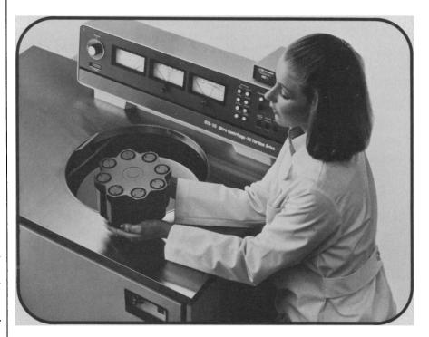
Sorvall® OTD ultracentrifuges with oil turbine drive and Automatic Rate Controller are ideal for density gradient work. The soft start and soft stop characteristics of the ARC and Reograd mode of deceleration prevent mixing of the gradient at speeds between 0 and 1,000 rpm.
