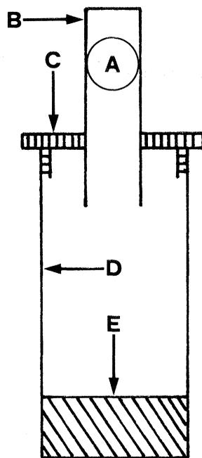
Fig. 1. Hydrogen sulfide test tube: sulfide-sensitive paper (A), small glass tube (B), polyethylene cap (C), large glass tube (D) containing the solution to be analyzed (E).
