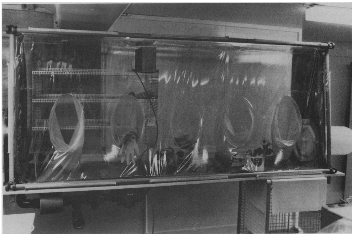
Fig. 1. Photograph of an Elster isolator measuring 2.5 m long, 0.7 m broad, and 1 m high. It is made of a flexible (though resistant) transparent plastic sheet held by a tubular frame, set up on a table with filters and machinery attached underneath. There are five regularly spaced gloves along the front, which permit manipulation in all parts of the internal volume. The isolator is maintained under negative pressure (which can be varied from 0 to -7 mm of water). The incoming and extracted air is passed through Hepa filters. Because of the limited air flow, these filters will last for many years. There are two circular openings, one on each side. The biggest one, on the left, is for taking in or out large sized equipment. The other, which is the transfer system door, shown here with a container plugged in, is used to take materials in or out during experiments. When the container with its lid is applied onto the transfer door and rotated, it triggers the isolator's door which can now be opened from inside. The lid of the container is stuck to the door in such a way that the external faces of both the lid and the door are protected from contamination. The tightly closed container can be transferred to another isolator or autoclaved (with metal containers not shown). The inlet for formol or peracetic acid is at the bottom left. The internal volume is closed and remains safe even if air extraction stops. Since plates may have to be incubated or cultures grown at temperatures ranging from 30° to 40°C, the entire isolator is thermally regulated, and the internal temperature can be varied at will. Plates are incubated on the bench, and cultures are grown on a shaking platform. A magnetic stirrer is available for cultures of 1 to 2 liters, and a small electric pump can be used to bubble air through the culture. Samples could be subjected to ultracentrifugation by sealing the opening of the ultracentrifuge in the same or another isolator while the centrifuge itself remains on the outside.
