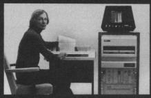
Quantex-Ray is a completely computerized X-ray energy spectrometer system for rapid quantitative elemental analyses. It's an enormously flexible system, allowing both interactive and automatic operation. In fact, operation can be so automatic that all you do is type one simple command to activate a total analysis. What does Quantex give you? In one, totally modular XES system, Kevex provides:
