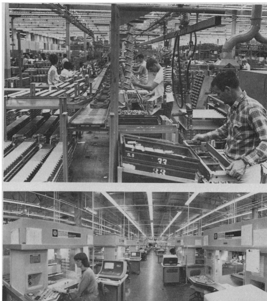
Fig. 5. (Top) An assembly line for crossbar switches at Western Electric's Oklahoma City plant. The assembly line typified the electromechanical crossbar technology of 15 years ago. (Bottom) Assembly area of Oklahoma City plant today. The operation illustrated is the wiring of grids on multilayer printed circuit boards. [Source: Western Electric Company]
