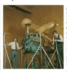
In another study, we are using signal coherence analysis to relate cylinder combustion pressure to noise radiation. This is part of an overall effort to learn in detail how engine structures transmit combustion-related noise.
