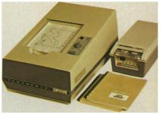
You can get clean, sharp, hard copies from the 4631 Hard Copy unit; local storage with the 4923 Digital Cartridge Tape Recorder; and proven software packages that quickly get you into Graphics. Below: 4012 Computer Display Terminal and 4662 Plotter.
