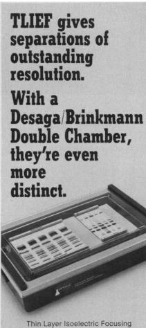
Thin Layer Isoelectric Focusing (TLIEF) is a new separation technique offering numerous advantages over conventional isoelectric focusing. These include simultaneous separation of multiple samples with outstanding resolution, accurate and simple pH determinations, and distinct evaluation by paper print technique.
