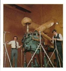
In another study, we are using signal coherence analysis to relate cylinder combustion pressure to noise radiation. This is part of an overall effort to learn in detail how engine structures transmit combustion-related noise.
