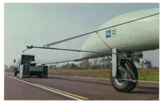
Considerable effort has been focused on tires, a major source of noise in both cars and trucks. Interestingly, air flow around the tire is not a significant noise source. But aerodynamic pumping between treads can be, depending upon tread pattern. Also important are tread vibrations in the vicinity of the contact patch.
