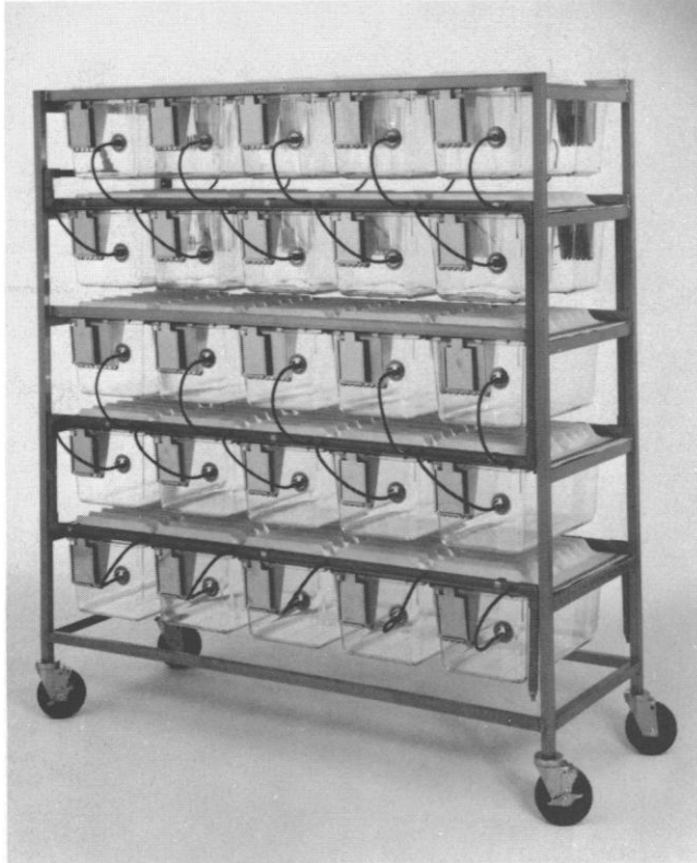
1. Mobile stainless steel rack with suspended polycarbonate cages.
