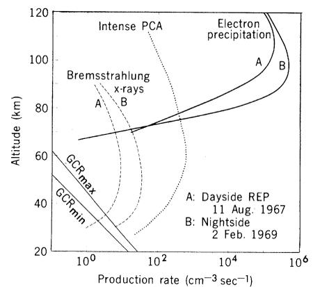
Fig. 2. Vertical profiles of the ionization (or NO production) rate during certain types of particle precipitation. The two solid lines below 60 km show the variability of GCR production over the solar cycle. The dotted line is an example of production during an energetic solar proton event characterized by intense PCA. Two examples of intense radiation belt electron precipitation are given including the production rate by the concomitant bremsstrahlung x-ray flux.
