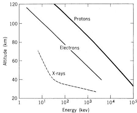
Fig. 1. The nominal penetration depth for energetic electrons, protons, and x-rays normally incident at the top of the earth's atmosphere.
