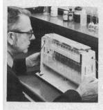
Suitable for both electrophoresing gels and destaining, the Model 1270 features a linear alignment of gel tubes and a bottom tank which can be easily lowered for access to all the tubes. Unlike circular units, this configuration does not require removal and emptying of the upper tank when changing tubes.
