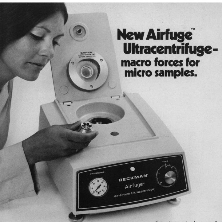
You're looking at a versatile new laboratory tool: a miniature, low-cost ultracentrifuge capable of speeds to 100,000 rpm and forces to 160,000 g.
