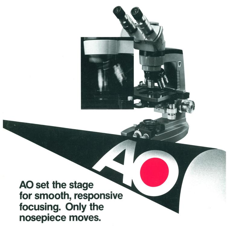
The AO® Series 10 MICROSTAR® Microscopes have a fixed stage. The focusing is done by moving the nosepiece.
