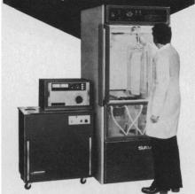
SAVANT'S HIGH VOLTAGE ELECTROPHORESIS ENCLOSURE WITH TWO LUCITE TANKS.
