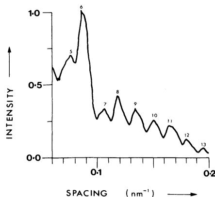
Fig. 2. Microdensitometer trace along the meridional direction of a low-angle x-ray diffraction pattern (the distance from specimen to film is approximately 10 cm) from an amianthoid area. Peaks correspond to diffraction orders (marked 5 to 13) from a periodic spacing of  $67 \pm 1$  nm; peaks of order  $< 5$  could not be recorded at this distance of specimen to film. The strongest recorded peak height is arbitrarily given a value of 1.
