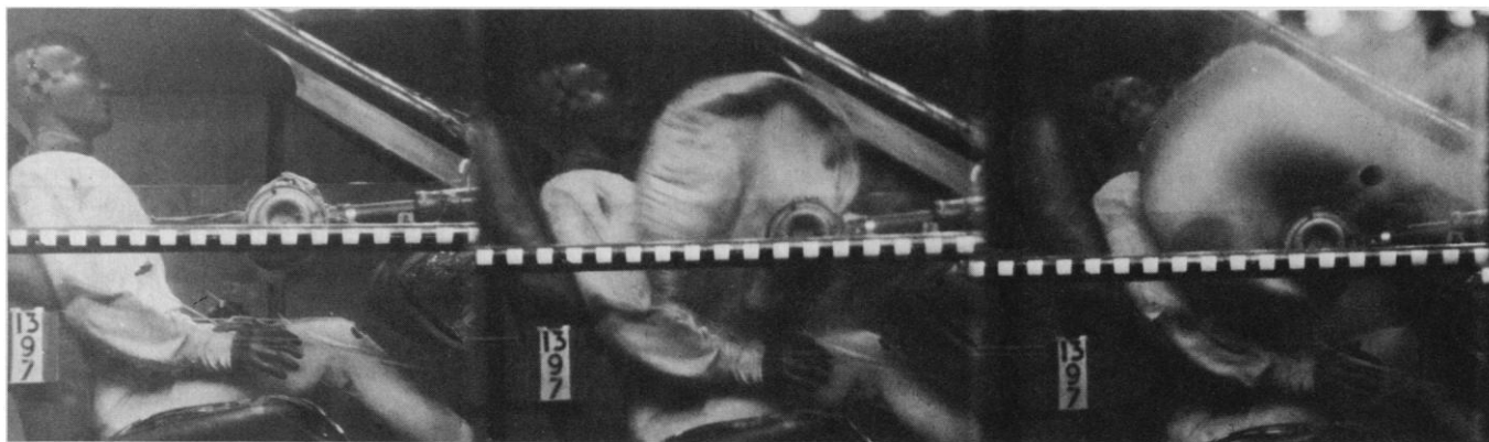
In this simulated crash at 47 miles an hour, the air bag starts to inflate and cushion the dummy 5 milliseconds after impact. The Calspan Corporation of Buffalo, New York, conducted the test on its high-energy impact machine.
