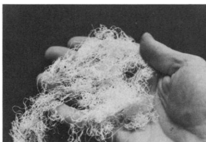
Fig. 1. Fibers of poly[bis(trifluoroethoxy)-phosphazene] prepared by solution extrusion into a nonsolvent.
