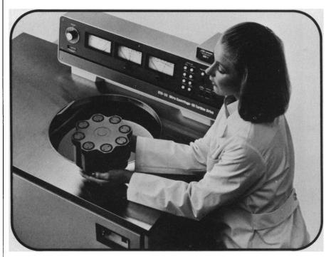
Sorvall<sup>®</sup> OTD ultracentrifuges with oil turbine drive and Automatic Rate Controller are ideal for density gradient work. The soft start and soft stop characteristics of the ARC and Reograd mode of deceleration prevent mixing of the gradient at speeds between 0 and 1,000 rpm.
