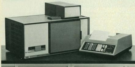
HP 5840 A Reporting Gas Chromatographs with microprocessor control of internal and external events permit ready automation of difficult analytical procedures.
