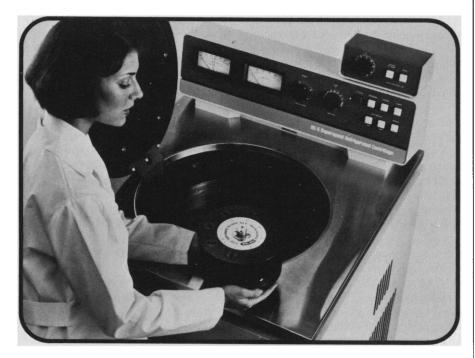
The Sorvall<sup>®</sup> RC-5 refrigerated superspeed centrifuge with a Rate Controller is ideal for density gradient work. The soft start and soft stop characteristics of the Rate Controller prevent mixing of the gradient at speeds between 0 and 1,000 rpm.
