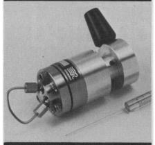
Use the new Rheodyne Model 7120 Syringe Loading Sample Injector Valve in two ways. Use it to fill loops conventionally for maximum precision or in the partial loop variable volume filling mode with only 0.5 microliter sample loss.
